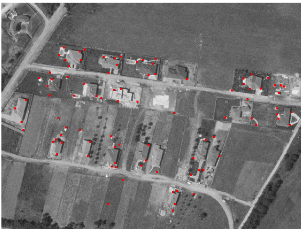
Figure 2.17: Remaining change keypoints after filtering with local contour descriptors.
