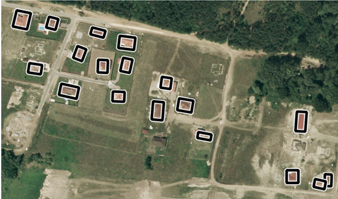
Figure 3.9: Rectangular footprint results, obtained by the MPP based detector module [72].
