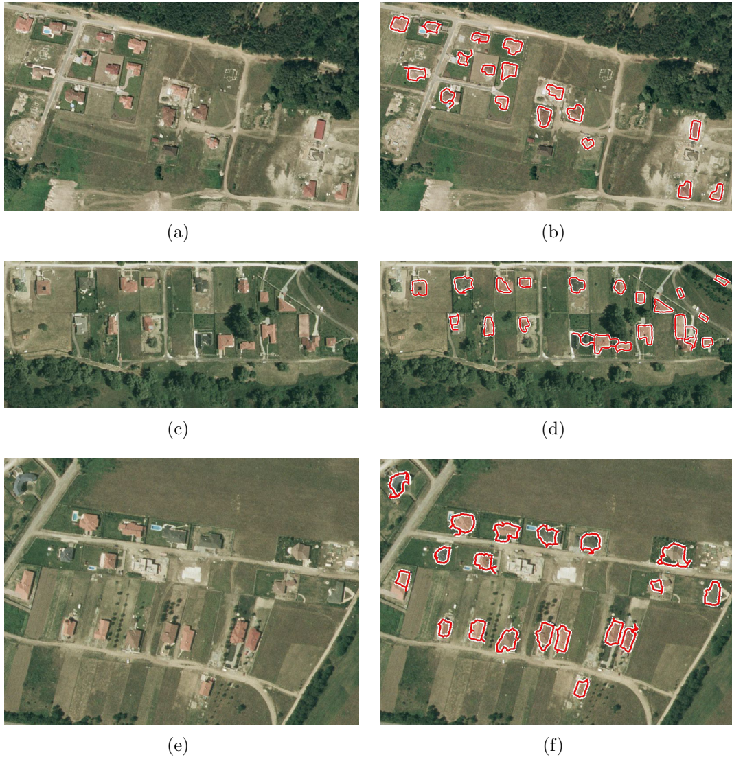
Figure 3.12: Results of the joint building localization and outline extraction approach. In the first column the original images can be seen, the second column shows the detected buildings.
