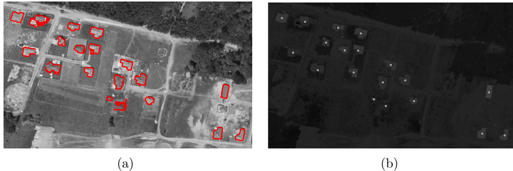
Figure 4.12: Result of the building detection with one main direction: (a) shows the detected contours; (b) is the estimated locations of the detected buildings.
