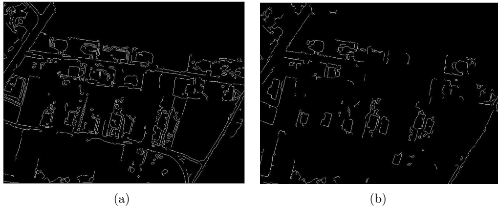
Figure 2.20: Result of Canny edge detection on different colour components: (a) is for R component of RGB space; (b) is for u^* component of L^*u^*v^* space.
