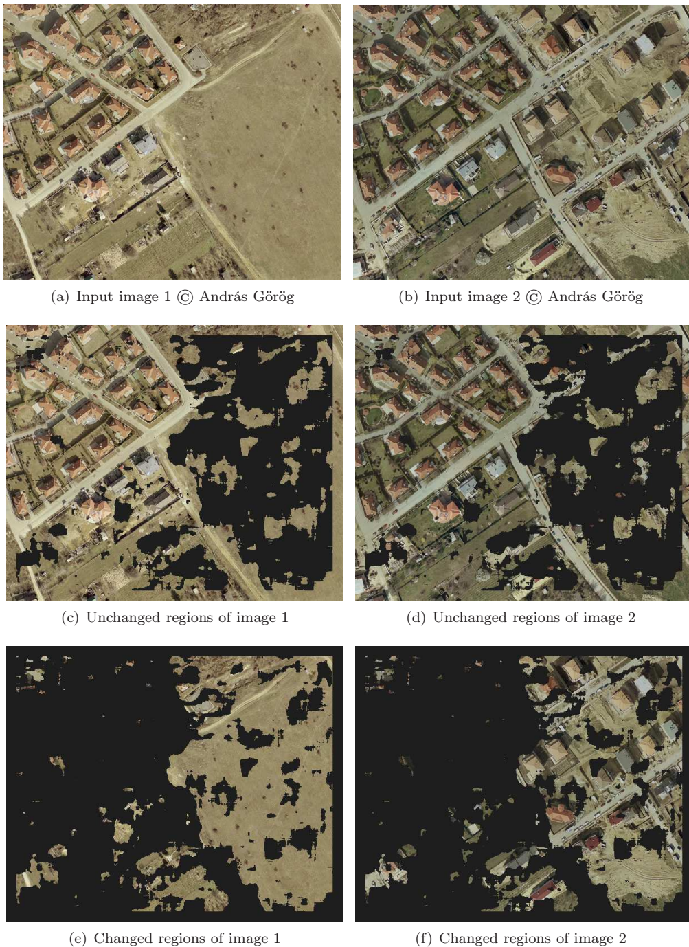
Figure 14: Detected changes with the Bhattacharyya distance, BUDAPEST image pair © András Görög. (c) and (d) show the unchanged areas, (e) and (f) present the change mask overlay on images 1 and 2
