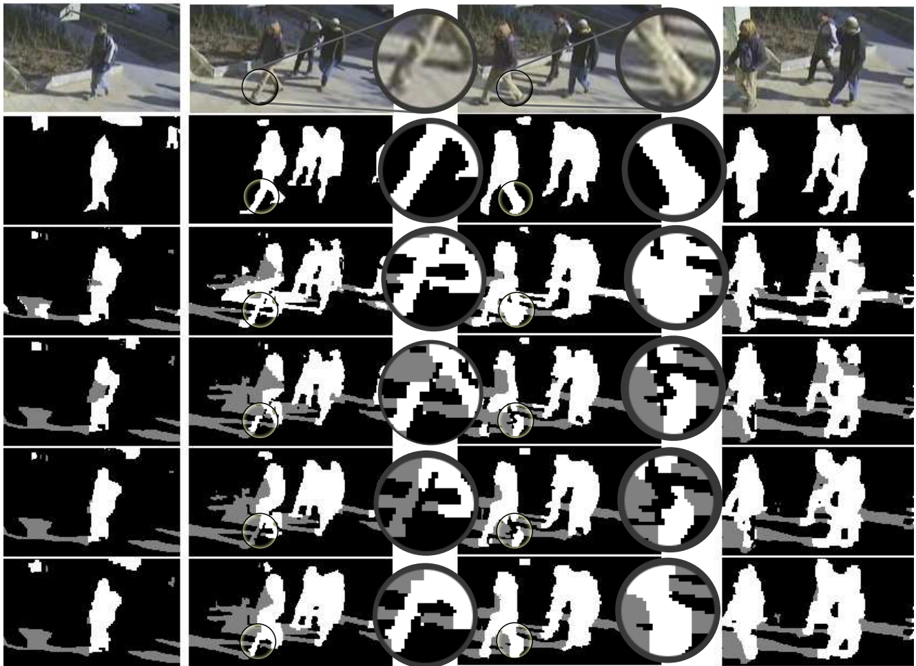
Fig. 8. Validation of all improvements in the segmentation regarding 'Entrance pm' video sequence Row 1. Video frames, Row 2. Ground truth Row 3. Segmentation with the 'constant ratio' shadow model, Row 4. Our shadow model with 'uniform foreground' calculus Row 5. The proposed model without microstructural features Row 6. Segmentation results with our final model.
