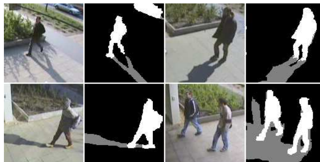
Fig. 3. Different periods of the day in the ‘Entrance’ sequence, segmentation results. Above left: in the morning (‘am’), right: at noon, below left: in the afternoon (‘pm’), right: wet weather.
