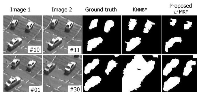
Fig. 9. Comparison of the proposed  $L^3$ MRF model to the KNNBF method, using image pairs from the KARLSRUHE sequence (# denotes the frame number). In consecutive frames of the video (above) KNNBF produces better results, however, our  $L^3$ MRF model significantly dominates if (below) we chose two frames with 1 second time difference
