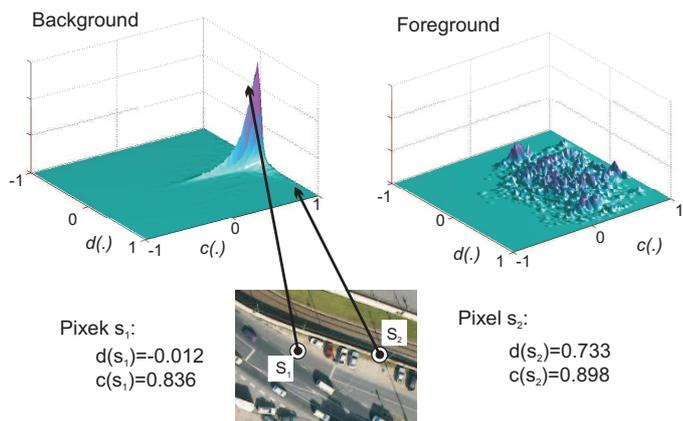
Fig. 11. Limitations of the observation fusion approach with the proposed feature selection. Above: 2-D joint histogram of the  $\bar{f}(s) = [d(s), c(s)]$  vectors obtained in the background and in the foreground training regions. Below: two selected *background* pixels and backprojection of the corresponding feature vectors to the background histogram.
