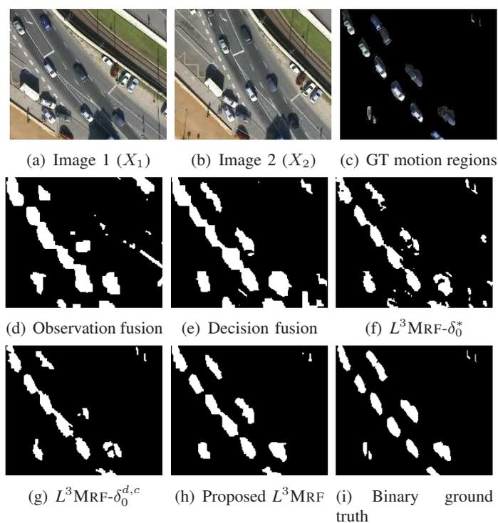
Fig. 12. Evaluation of the proposed  $L^3MRF$  model versus different fusion approaches. Methods are described in Section -A.
