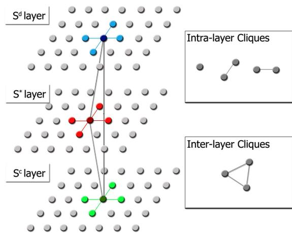
Fig. 4. Structure of the proposed three-layer MRF ( $L^3$ MRF) model
