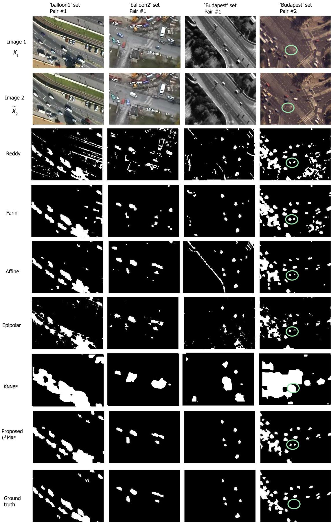
Fig. 6. Comparative segmentations: four selected test image pairs, segmentation results with different methods and ground truth. In the right column, the ellipses demonstrate a limitation: a high standing lamp is detected as a false moving object by all methods.
