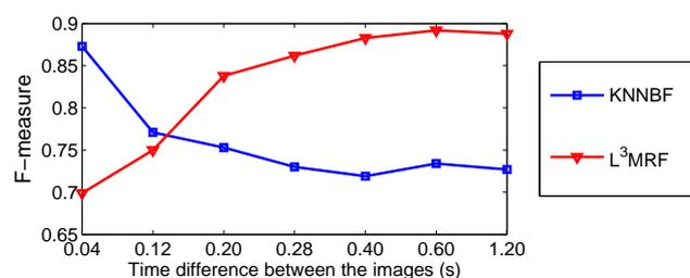
Fig. 10. Comparing KNNBF to  $L^3$ MRF. Quantitative segmentation results ( $F$ -measure) of different frame pairs from the KARLSRUHE test sequence, as a function of the time difference between the images. The proposed method dominates if the images are taken with larger elapsed time, which results in large object displacements.
