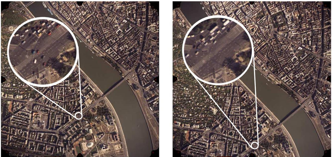
Fig. 1. High resolution stereo image pair taken by the Hungarian Ministry of Defence Mapping Company<sup>©</sup> above Budapest with a few sec. time difference.
