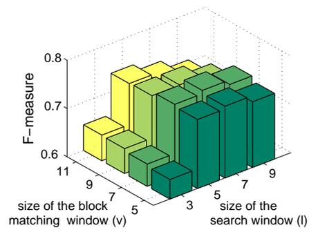
Fig. 5. Performance evaluation as a function of the block matching ( $v$ ) and search window size ( $l$ ) using training images from the ‘balloon1’ test set. Here,  $v = 7$  and  $l = 7$  proved to be optimal.
