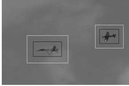
**Fig. 4:** The inner (darker color) rectangles represent the bounding boxes of the detected edge and corner points. Pixels outside the inner rectangles are used for *training* the global background model. Pixels outside the outer rectangles (lighter color) are always classified as background in the preliminary segmentation step.
